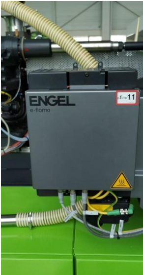
Illustration of a distribution box with customer-specific designation (11)
